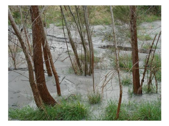
Failure of embankment of Waimakariri river due to liquefaction of its surroundings. Lateral spreading assisted
